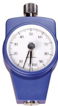
Figure 2.9: The shore hardness tester Analogue Shore Scale “D” type Durometer.
