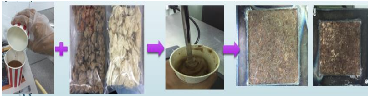
Figure 3.8: Sample preparation of fibre composite.
