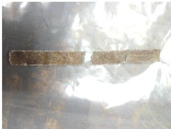
Figure 4.7: Flexural test on untreated fibre composite
