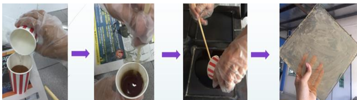
Figure 3.7 : Sample preparation of neat polymer.
