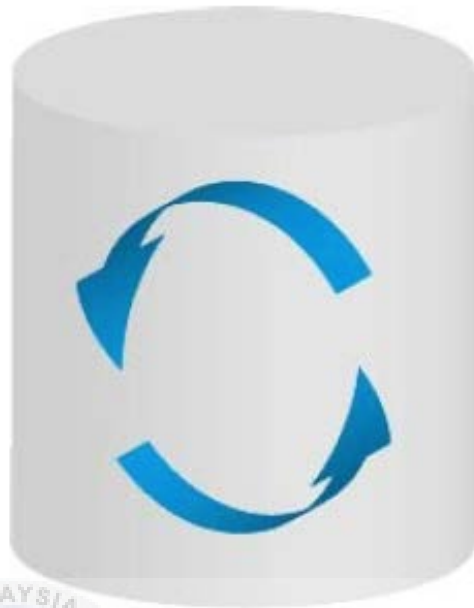
Figure 2.9: In-cylinder Tumble motion
