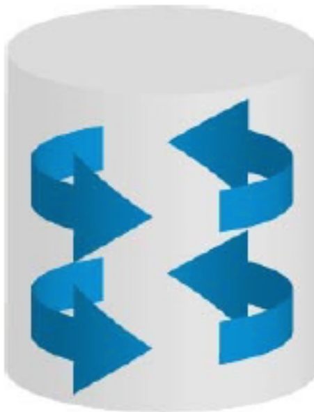
Figure 2.5: In-cylinder swirl motion
