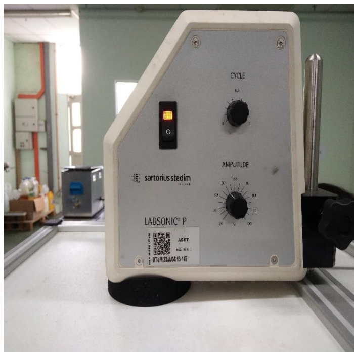
Figure 3.4 : The setting used for the sonication is 0.5 in cycle and 50 Hz in amplitude
