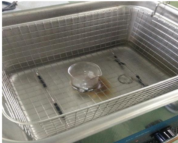
Figure 3.7 : Steel ball being clean with the ultrasonic bath machine
