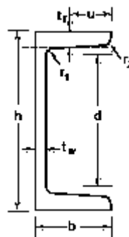
Figure 2.3 : Cross Section of Mild Steel Channel
