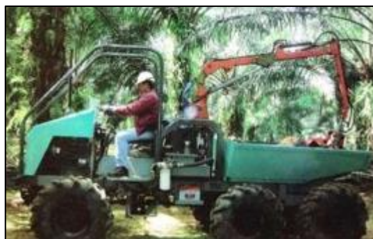
Figure 2.1 : Current 6x6 oil palm fruit bunch utility transporter
