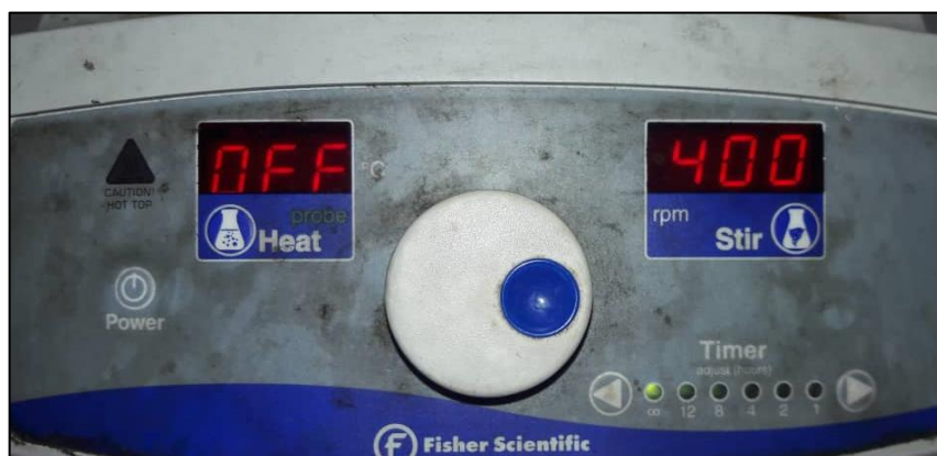
Figure 3.5: Setting the rotation per minute to 400 RPM
