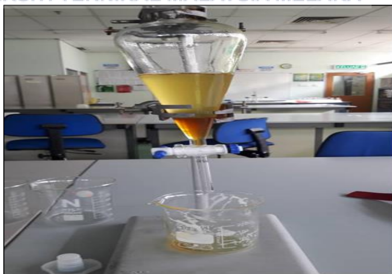
Figure 3.8: Separation between Glycerin and Crude Fatty Acid Methyl Esters
