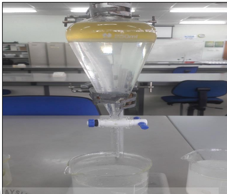
Figure 3.9: Fatty Acid Methyl Esters after washing process.
