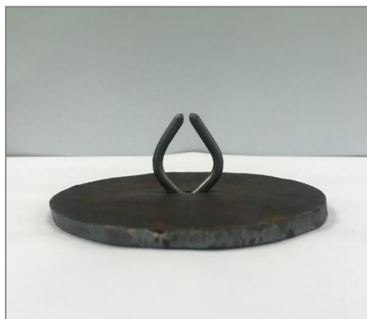
Figure 4.15: Corroded at 6 cm electrode length
