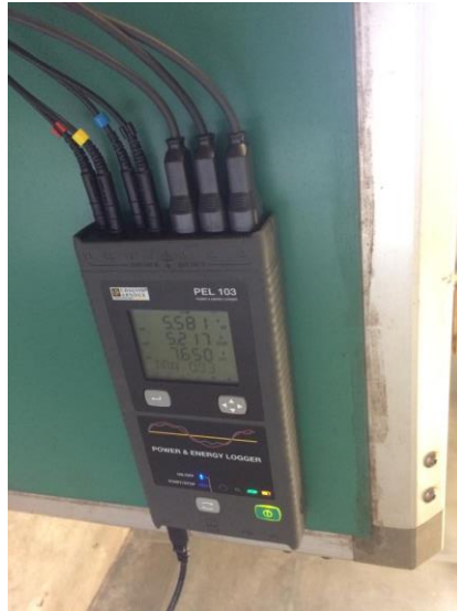
Figure 3-8: Power Logger Device
