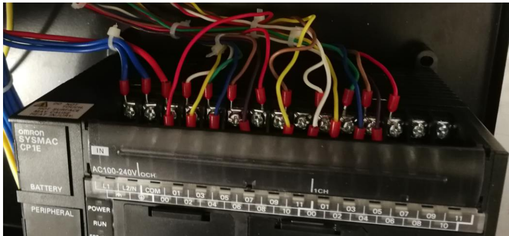
Figure 4.5 Input Signal from Conveyor Sorter System
