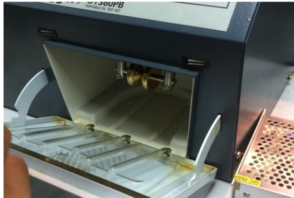
Figure 3-9 : 1mm gap of Megger OTS60PB
