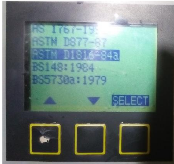
Figure 3-11 : Select ASTM D1816 standard
