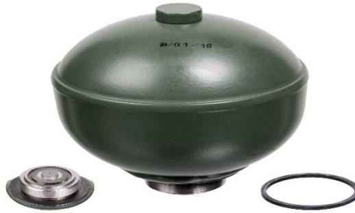
Figure 2.2: Hydro-pneumatic suspension (sphere)
