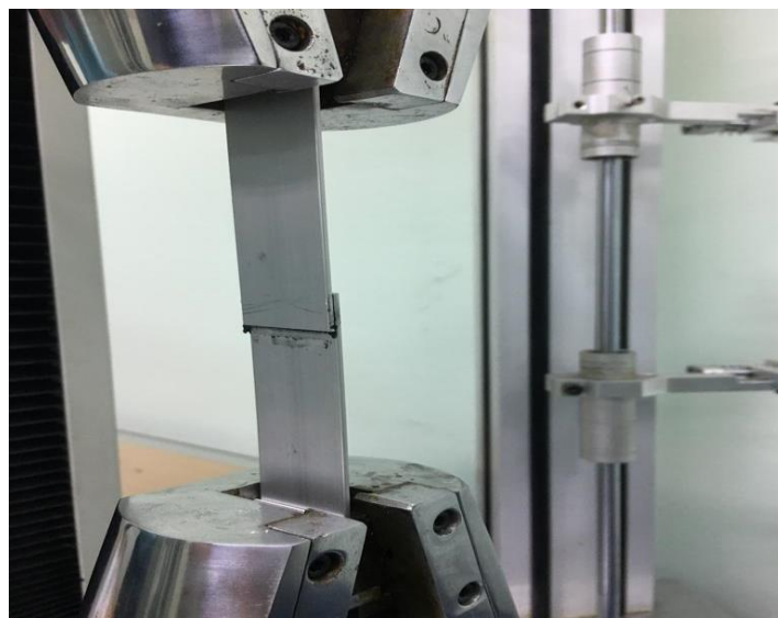
Figure 3.22: Lap shear testing test set up using a Universal Testing Machine, UTM.
