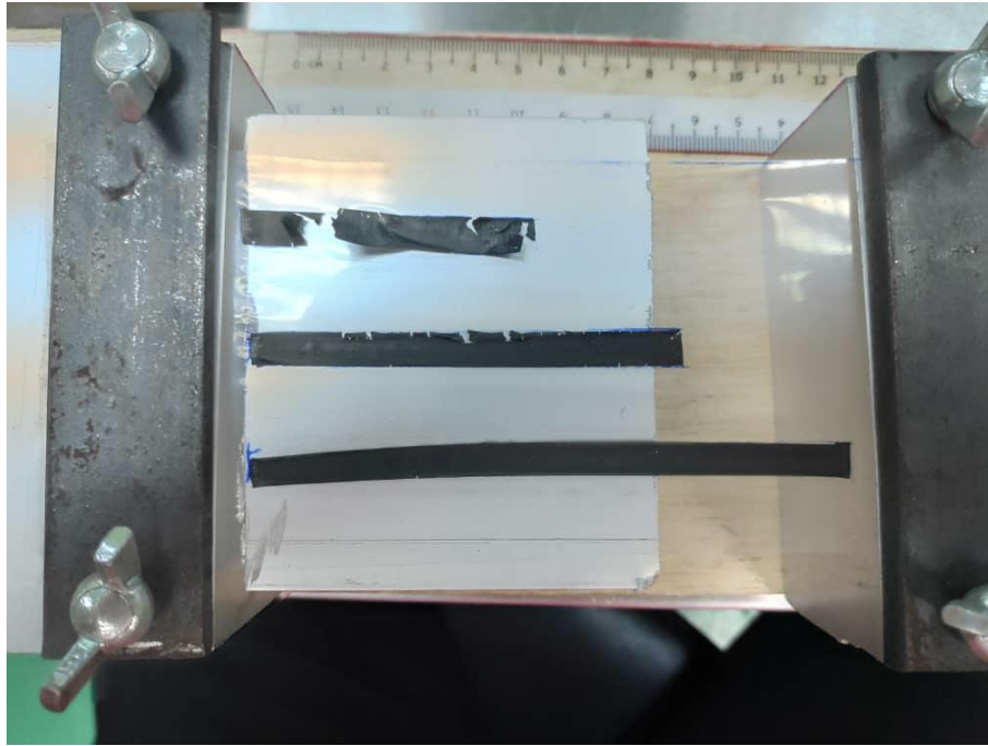
Figure 4.14: Crack of conductive ink with 60mm length (middle) when stretch with 28% of its total length.
