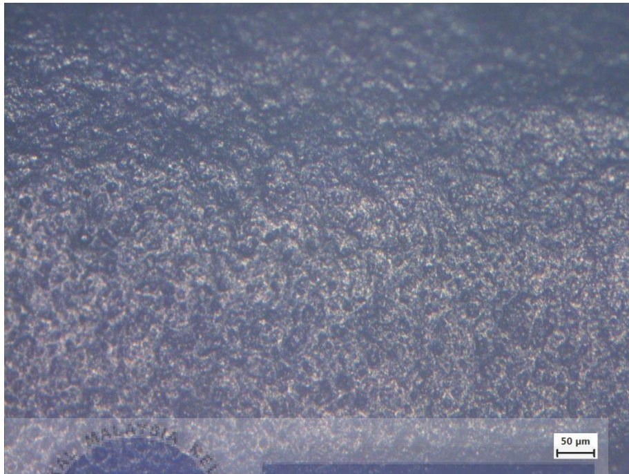
Figure 4.8: The microstructure of conductive ink (40mm length) before stretching.
