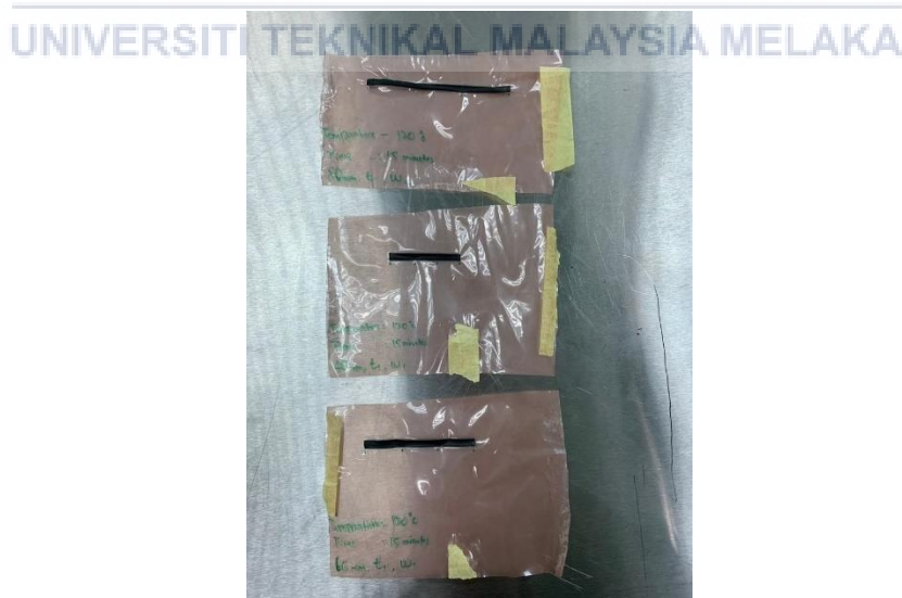
Figure 3.7: Remove the scotch tape after screen printing.
