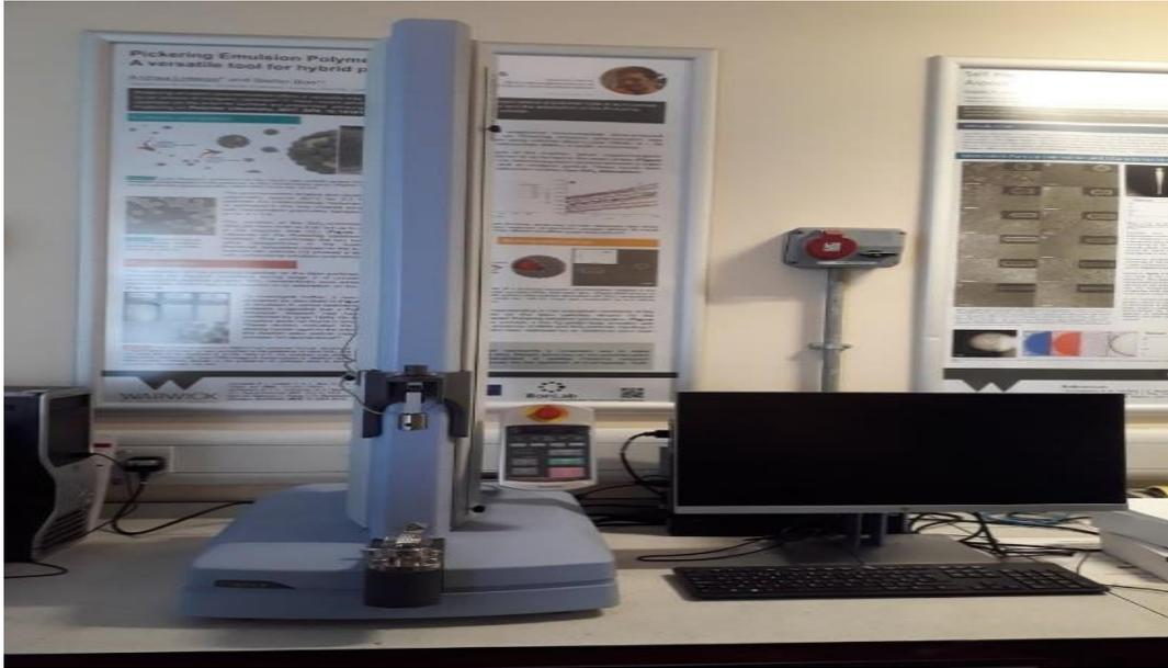
Figure 3.5.1: Shimadzu EZ Test (EZ-LX) test machine
