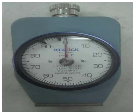
Figure 3.21 Durometer Test (in shore D)
