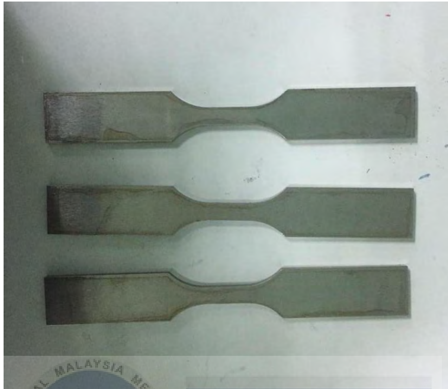
Figure 3.1 : Specimens of AISI 1045 Medium Carbon Steel
