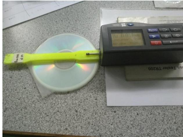
Figure 4.16: Sample of dog bone during surface roughness test
