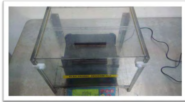
Figure 3.29: Take the reading density of POF/PP composites.
