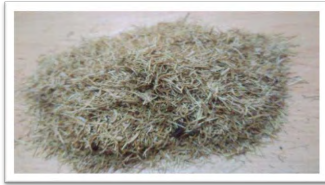
Figure 3.5: The POF was cutted less than 1 cm
