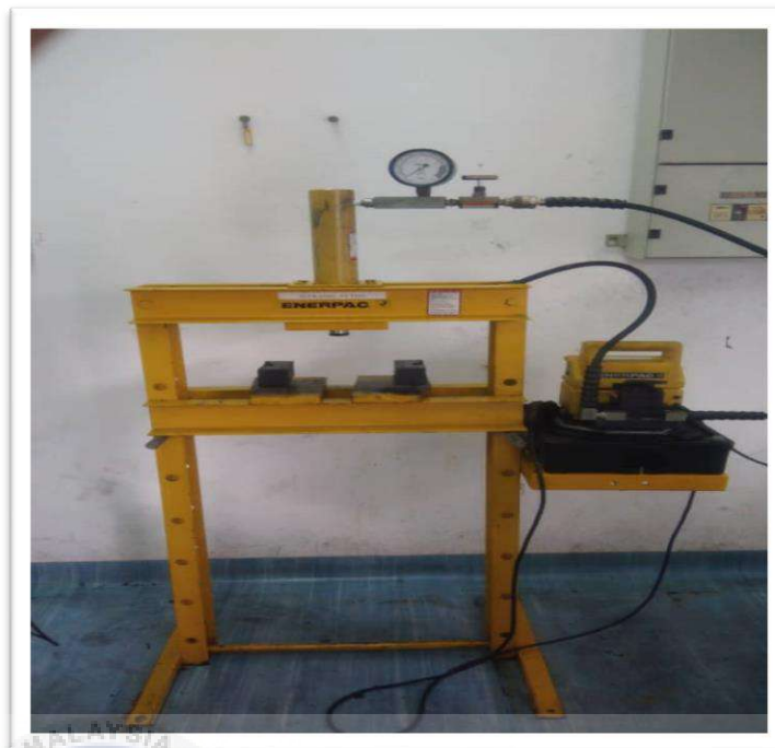
Figure 3.20:H-frame used to carry out the POF/PP composites
