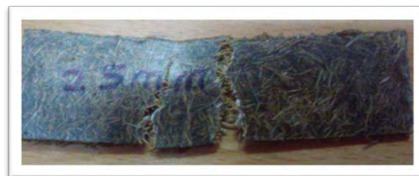
Figure 3.26: POF/PP composite samples ruptured after tensile test
