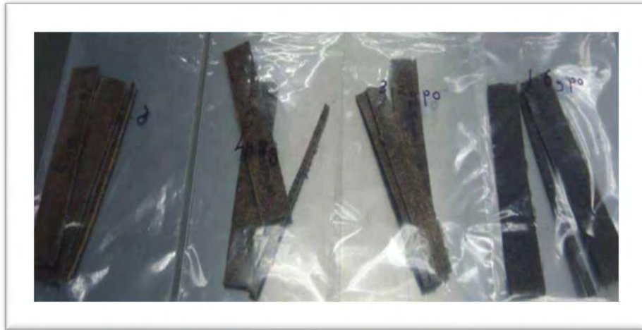
Figure 3.22: The POF/PP composites cutted to specific dimension.
