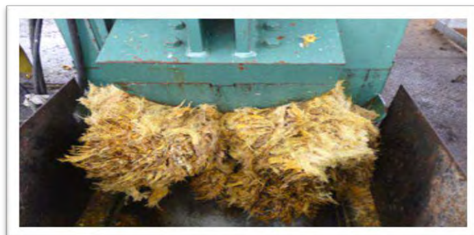
Figure 3.3: The machine crusher machine to extract POF from POEB
