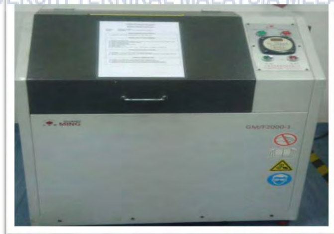
Figure 3.8: The pulverize machine to crush PP.
