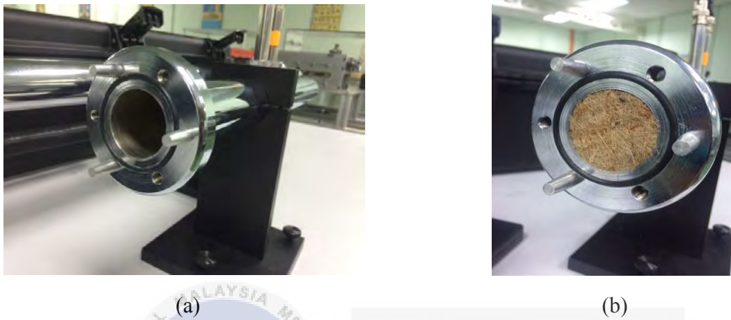
Figure 3.15: (a) The empty sample holder of impedance tube (b) The sample fitted into the holder
