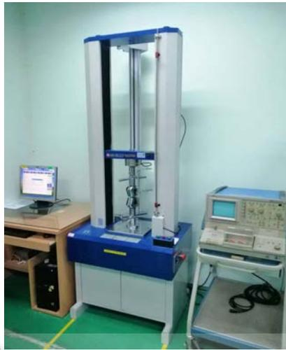
Figure 3.13 Universal material testing AG – 10kNX machine
