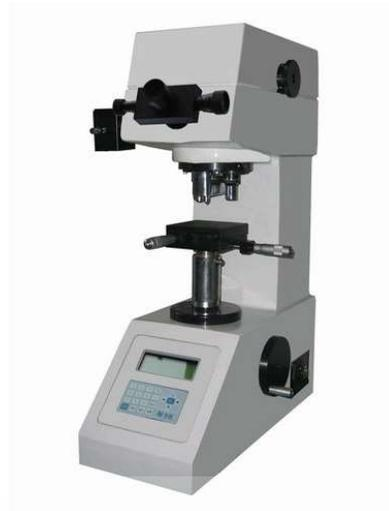
Figure 3.11 Vickers microhardness testing
