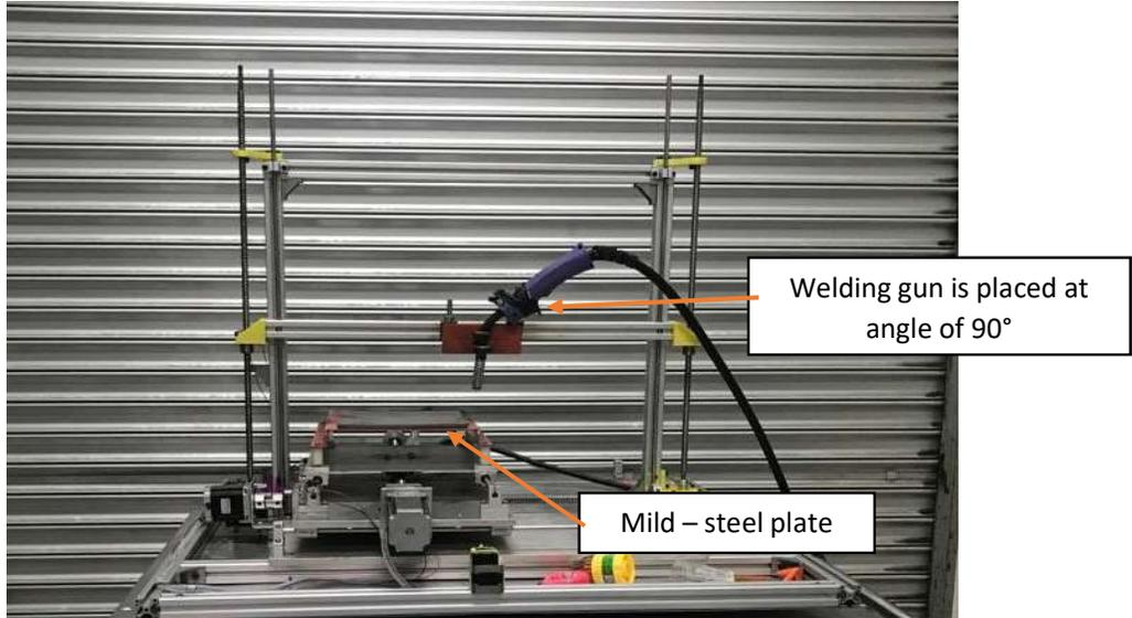
(a) WAAM experiment setup without thermoelectric cooling system
