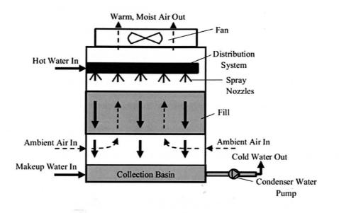
Figure 2.1 : Schematic of cooling tower
