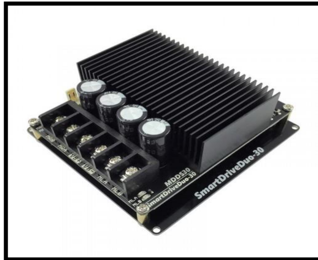
Figure 3.10: MDDS30 Motor Driver
