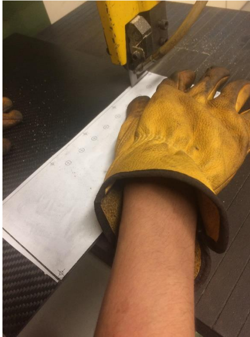
Figure 4.18 Cutting fuselage plates shape with band saw
