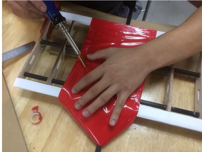
Figure 4.13 Iron plastic film onto surfaces
