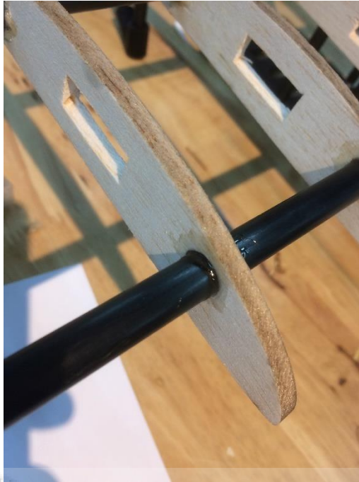
Figure 4.10 Ribs are glued onto the carbon fiber rod with epoxy
