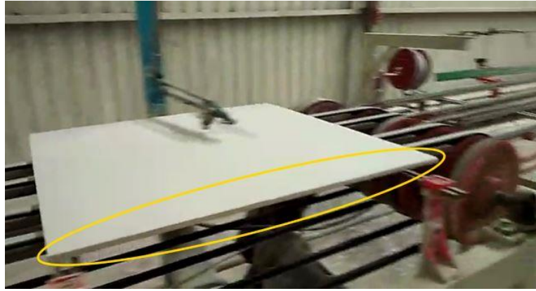
Figure 1.1: Quality Check of Tile Edge Defect [5]
