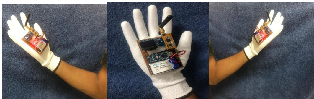
Figure 3.14 Hand orientation measurement device for hand
