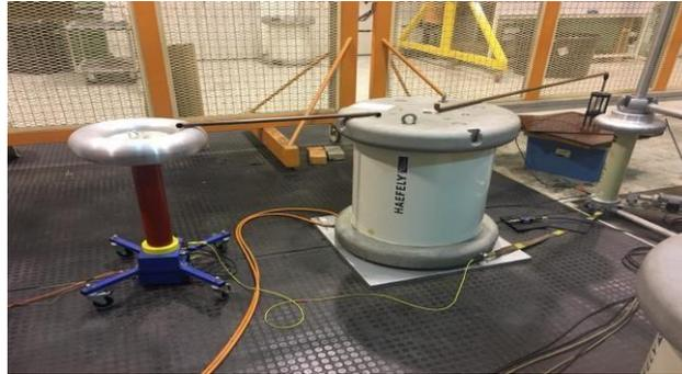
Figure 3.3 : Setup for PD experiment
