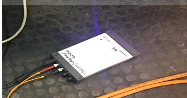
Figure 3.6 : The MPD600 detector
