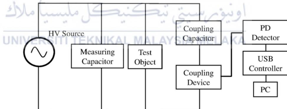
Figure 3.2 : Block diagram of PD measurement setup
