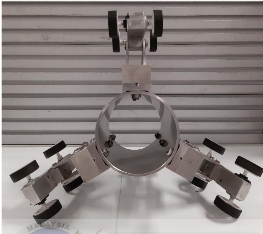
Figure 4.12: The Front View of the Fabricated Pipeline Inspection Robot
