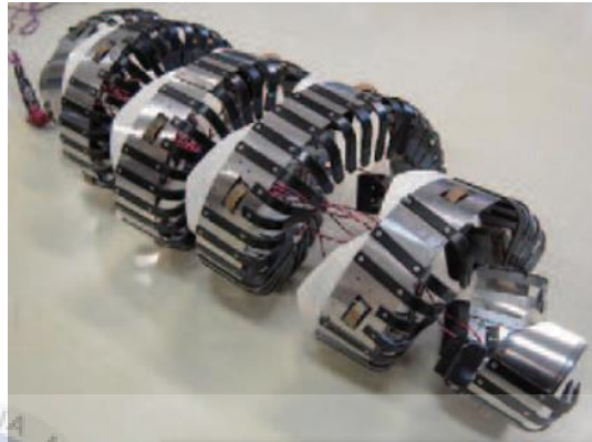
Figure 2.5: The Screw Type Robot Prototype SPRING by Osuka et al. [16]
