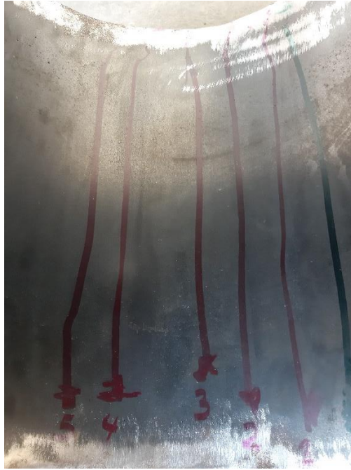
Figure 4.18: The Line Produced by the Pipeline Inspection Robot with 5 Trials
