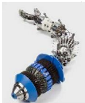
Figure 2.1: Pigs device that used in intelligent pigging method [14]
