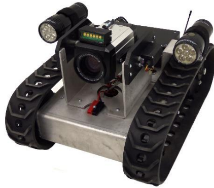
Figure 2.5: Caterpillar type robot with simple structure
