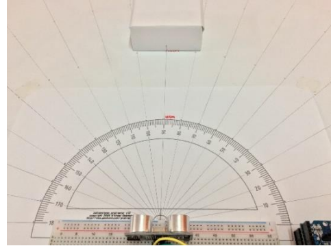
Figure 3.25: Obstacle 20cm far from the ultrasonic sensor
