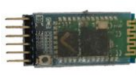
Figure 3.4: Bluetooth module HC-05
