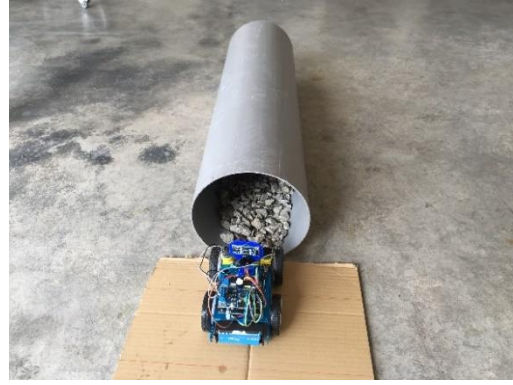
Figure 3.20: Set up of pipe with small stones
