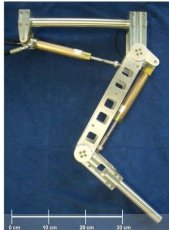
Figure 2.5 Picture of HYQ leg prototype with hydraulic cylinder, without compliant element and foot.[16]
