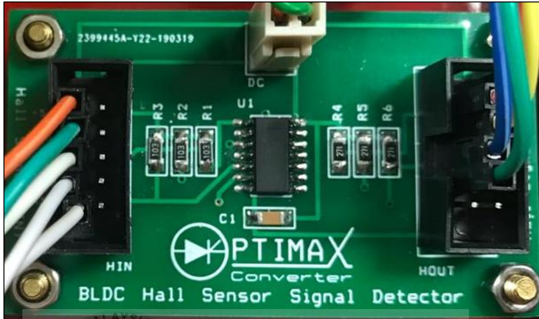
Figure 3.15: PCB of Hall Sensor Signal Detector
