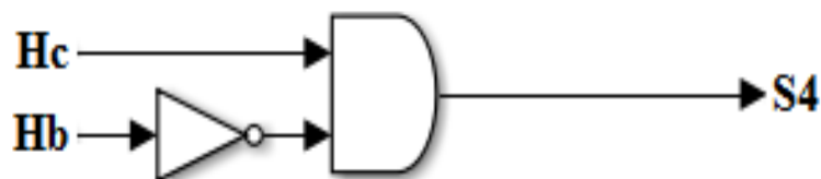
Figure 3.9: Logic Circuit for bottom IGBT of S4
