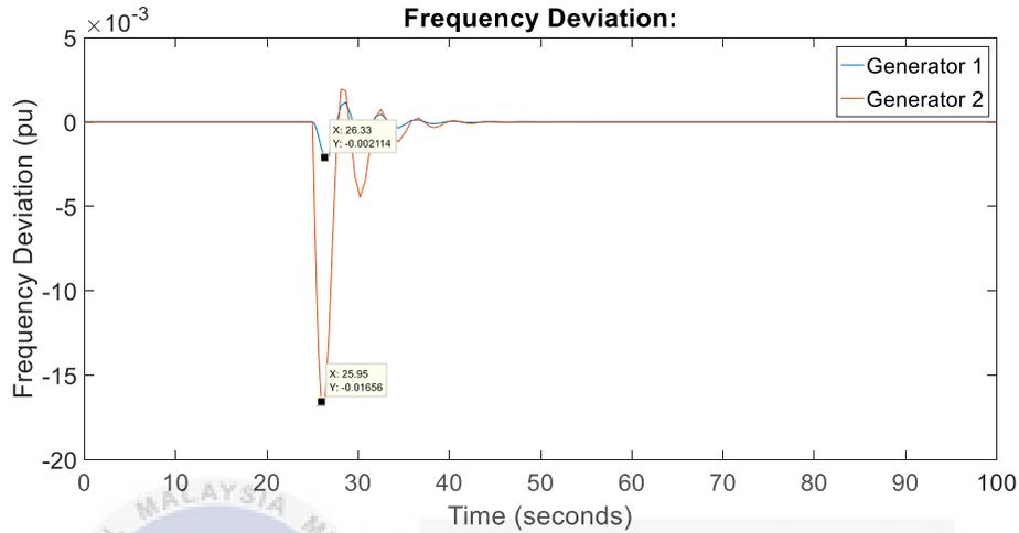
Figure 4.4: Frequency Deviation for Generator 1 and Generator 2
