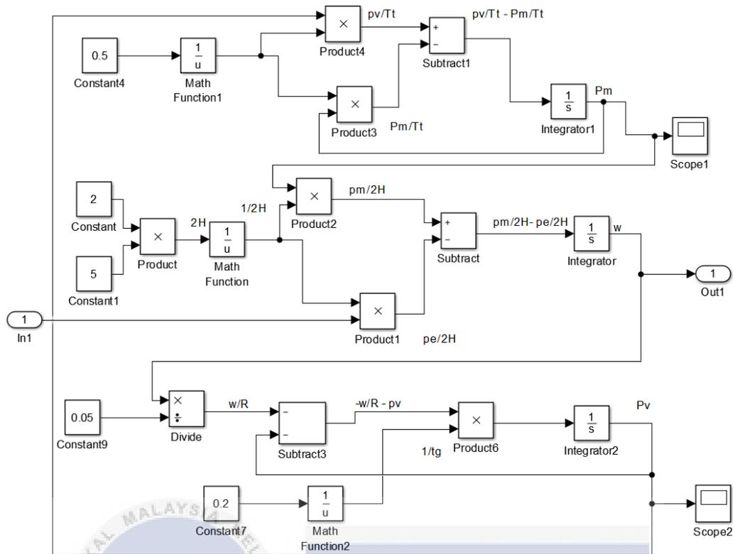
Figure 3.6: Simulation model of single generator
