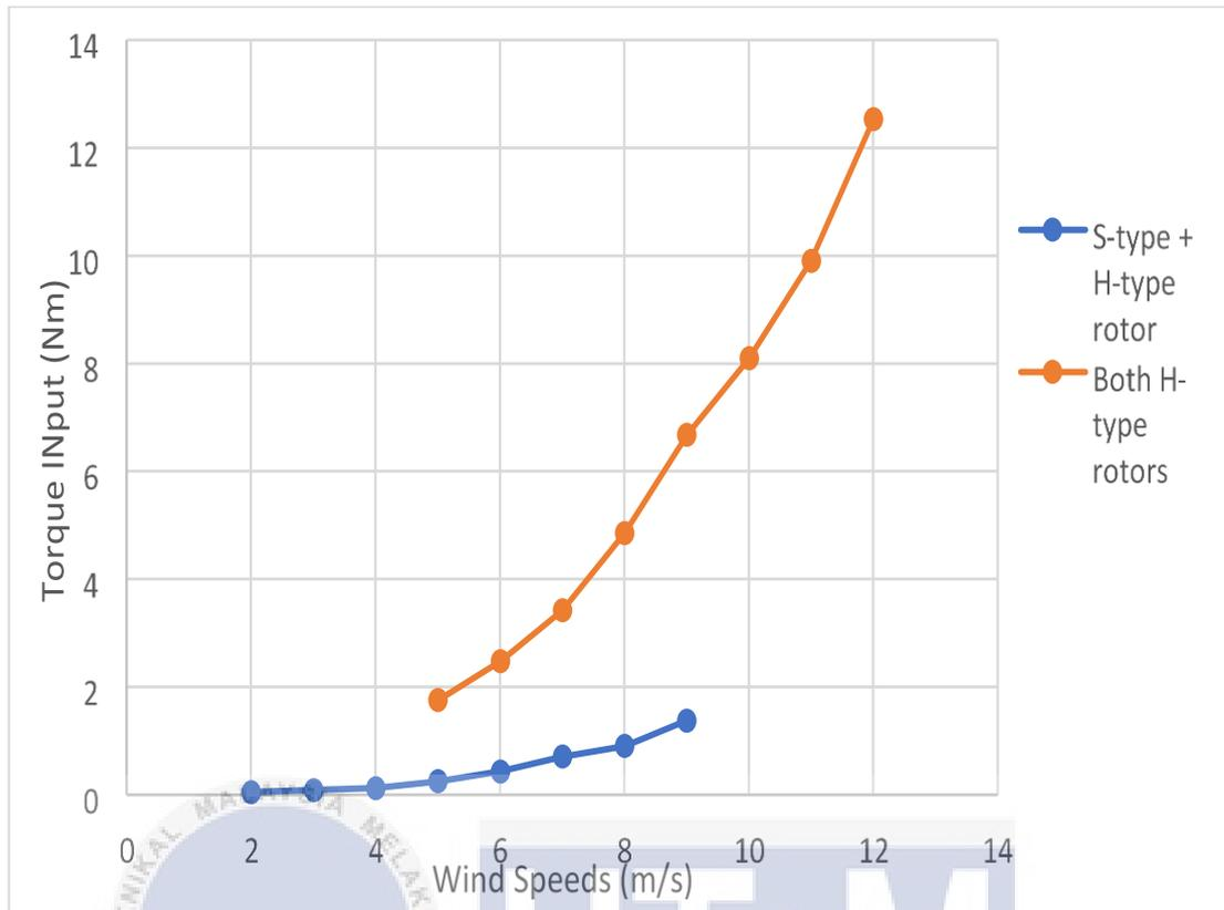
Figure 4.6: Comparison of torque input between CRWT of S-type and H-type rotor and CRWT of both H-type rotors
