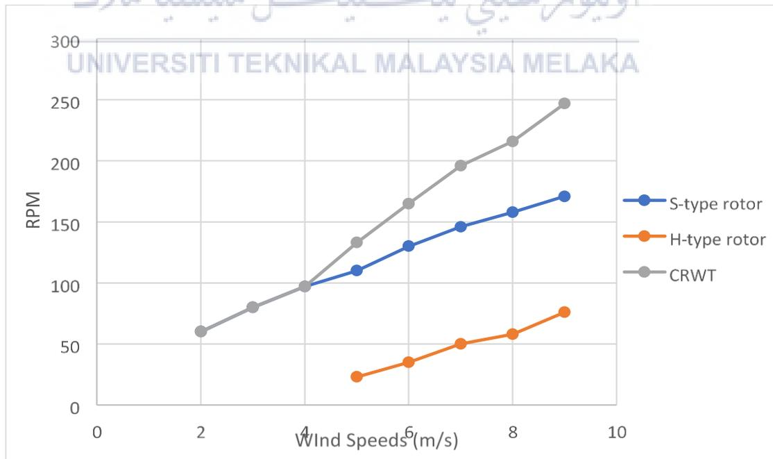
Figure 4.1: A variation graph of RPM for each rotor and CRWT system
