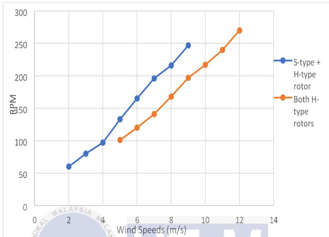
Figure 4.5: Comparison of rpm between CRWT of S-type and H-type rotor and CRWT of both H-type rotors
