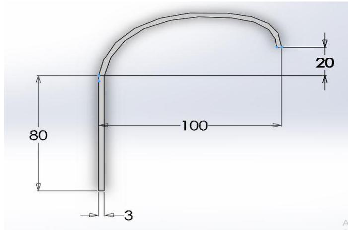
Figure 3.6 : Top view of S-type blade design
