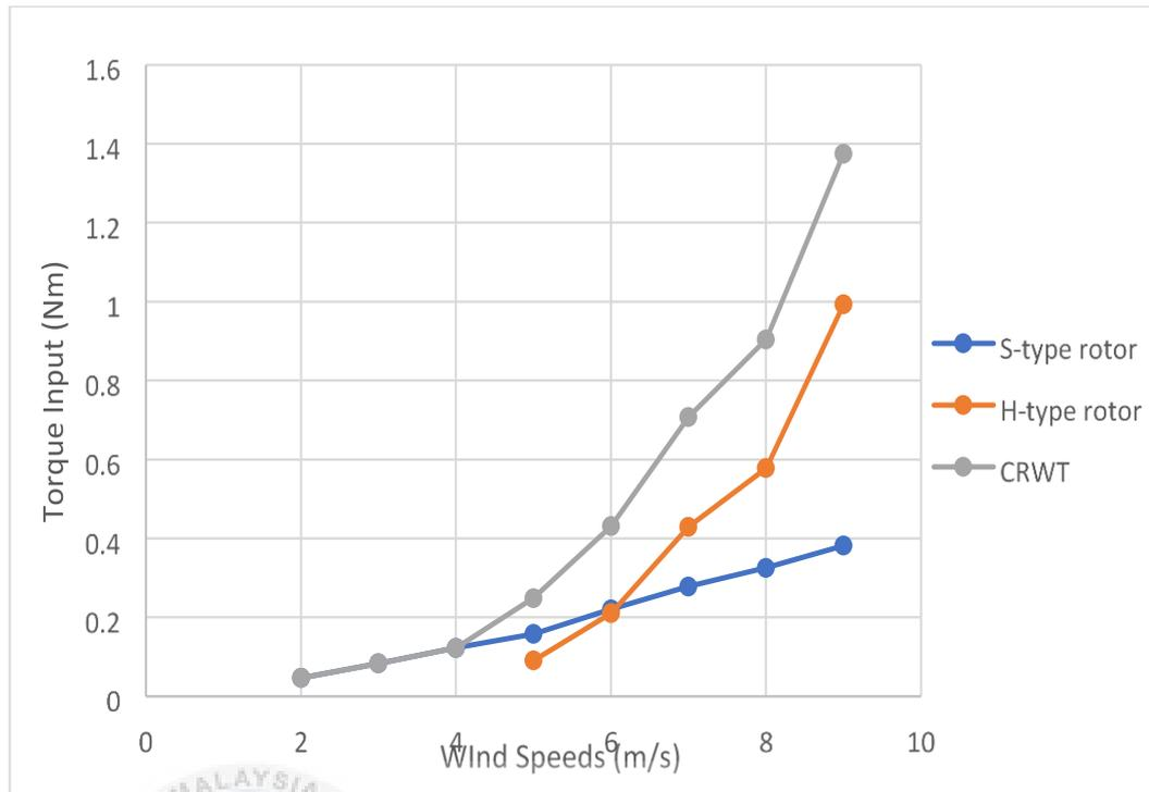
Figure 4.2: A variation graph of torque input for each rotor and CRWT system
