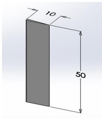
Figure 3.2 : Dimension of H-type blade design
