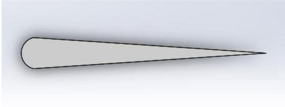
Figure 3.3 : H-type blade profile using NACA 0021airfoil
