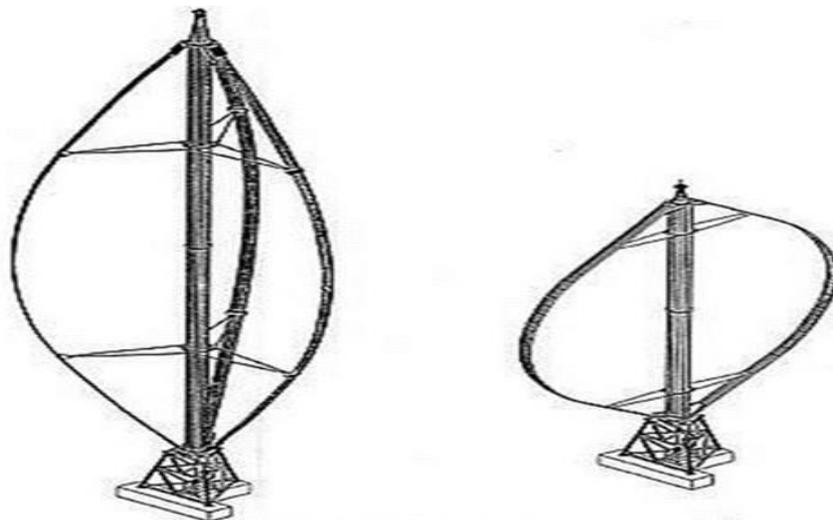
Figure 2.5: Darrieus-type wind turbine model [8]
