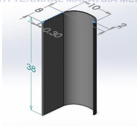
Figure 3.5 : Dimension of S-type blade design
