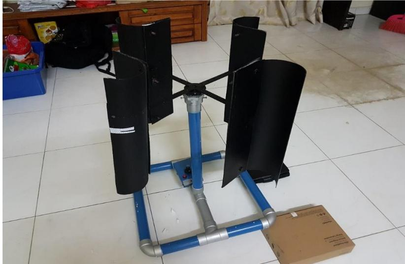
Figure 3.10 : S-type wind turbine
