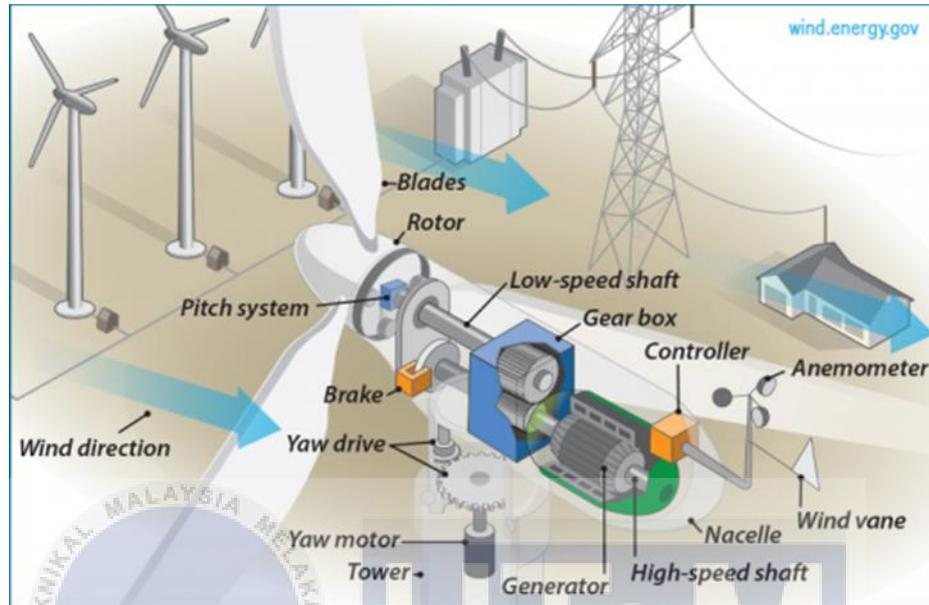
Figure 2.3: The wind turbine components [24]
