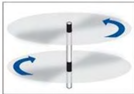
Figure 2.4 : The concept of counter-rotating wind turbine system [2]
