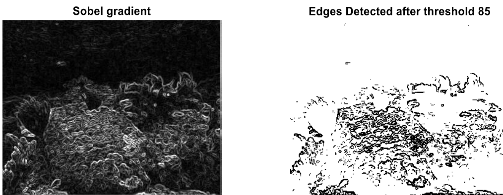
Figure 4-6: Edge detection of the image after color improvement
