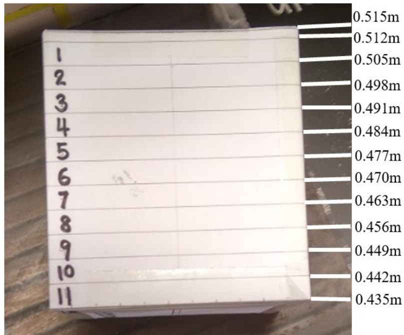
Figure 3.15: Top view of the tested object with its coordinate x_B when it is situated on the center point of the object (x_{obj}, z_{obj})
