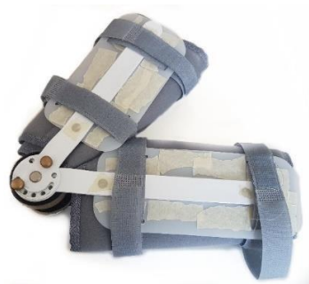
Figure 3.2 Elbow brace for simulated stroke
