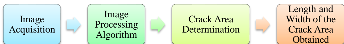
Figure 3.1 Overview of Underwater Pipeline Cracking Area Identification System
