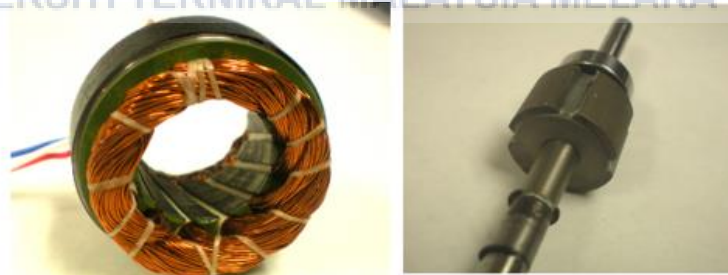
Figure 2.6: Brushless DC motor.
