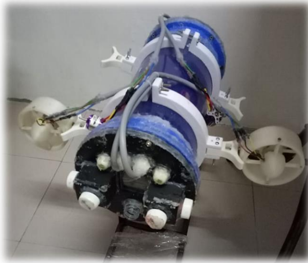
Figure 3.10: AUV design with the printing part.
