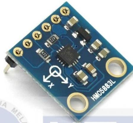
Figure 2.12: HMC5883L Magnetometer Sensor
