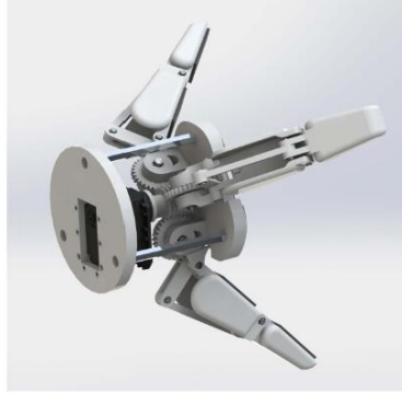
Figure 2.2 Worm wheel arrangement connecting to actuating worm in 3D view
