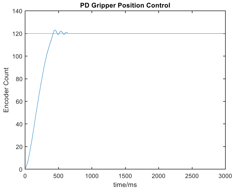
Figure 4.2 Output transient response of PD controller at 51.5^\circ
