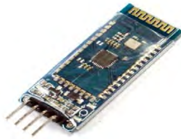
Figure 2.5: Bluetooth model HC-05 adapted from website mcuoneclipse by Erich Styger posted on June19,2015
