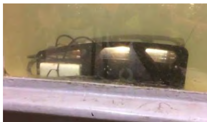
Figure 3.22: Waterproof test for AUV
