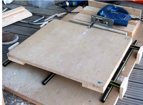
Figure 3.6: Shaking table using drill as actuator [34].
