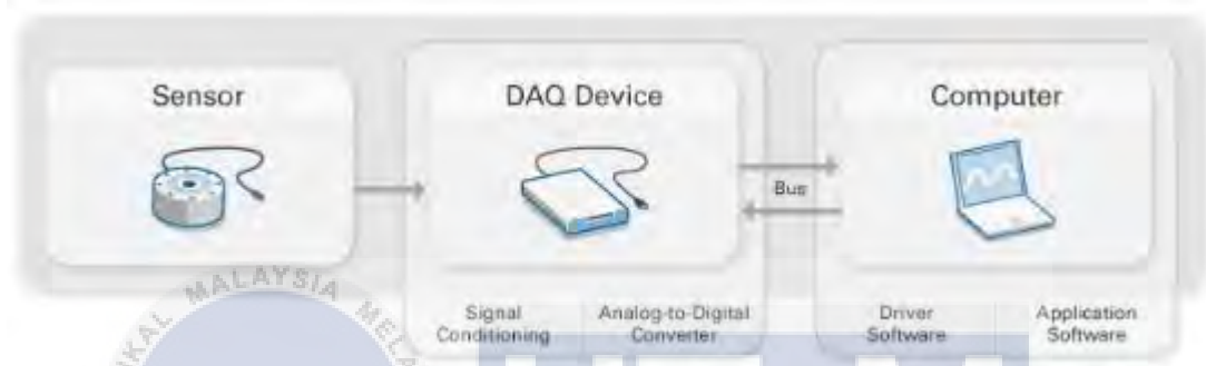
Figure 3.15: Block diagram of a measuring system [5]
