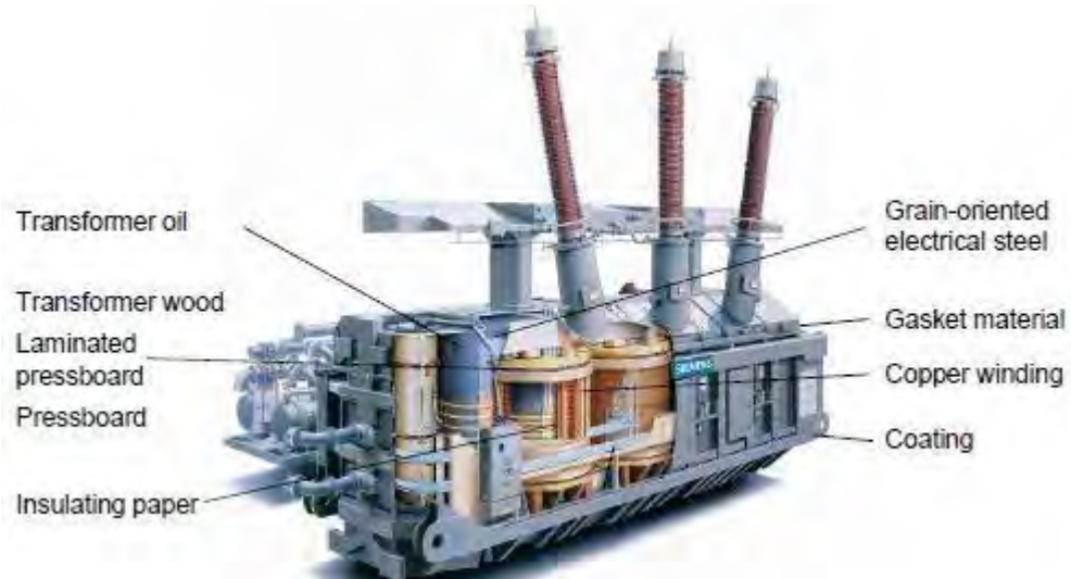
Figure 2.1: Structure of a transformer.
