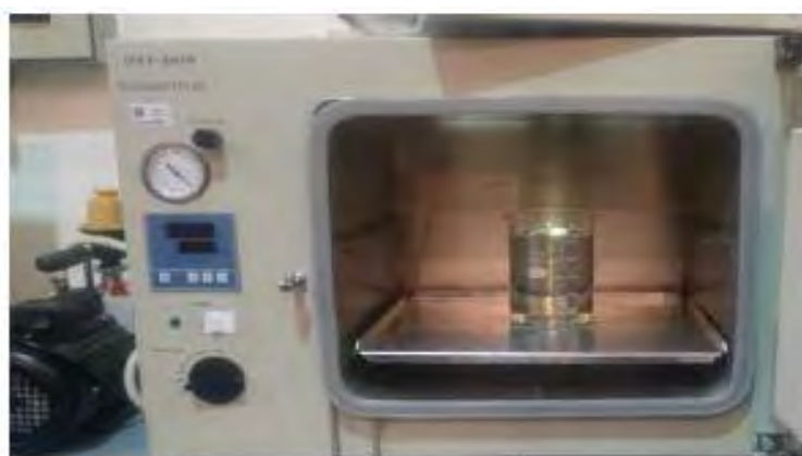
Figure 3.10: Placement of Sample in the Vacuum Oven (VO)
