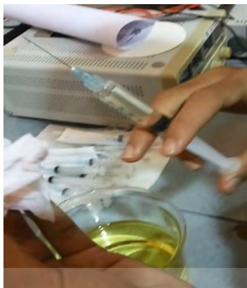
Figure 3.8: Syringes fill with oil sample
