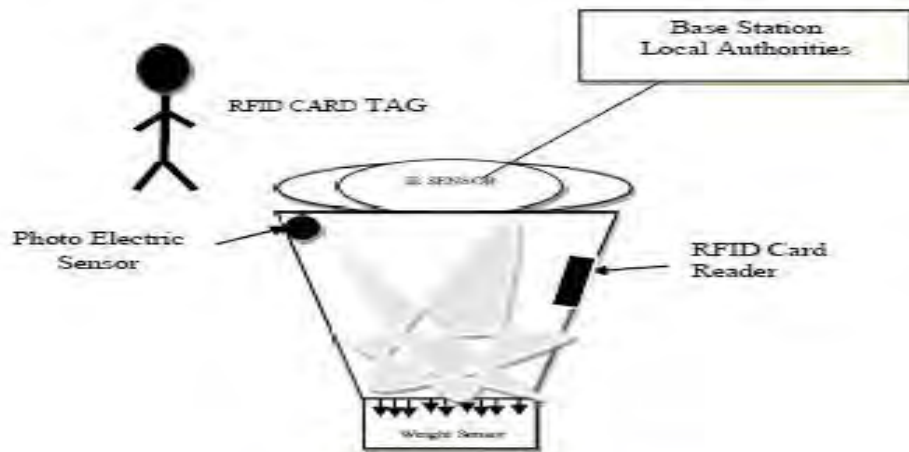
Figure 2.5 Block Diagram Of The System(M.Narayanan,2017)
