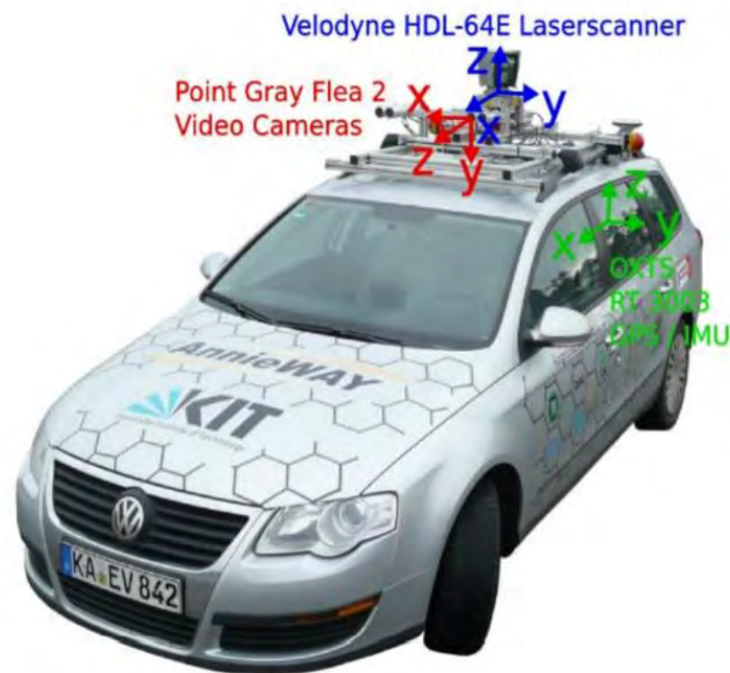
Figure 2.2.1: The sensor configuration on the platform
