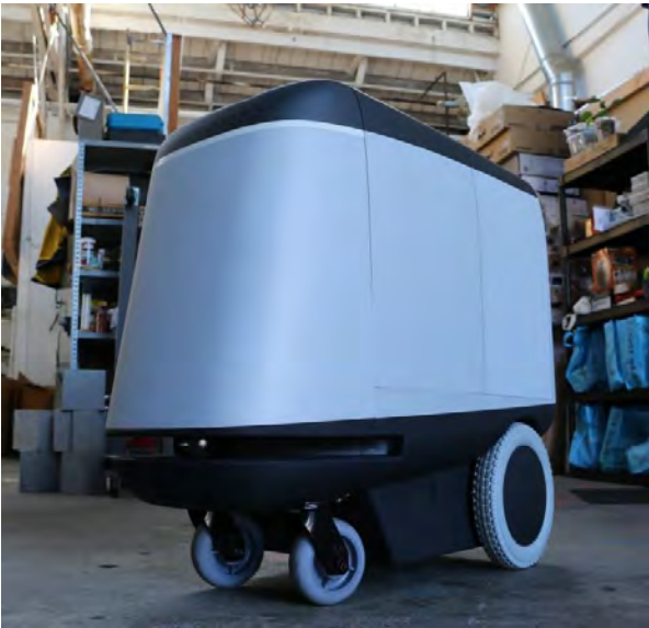
Figure 1.1 : AGV that use for delivering item in the industry warehouse
